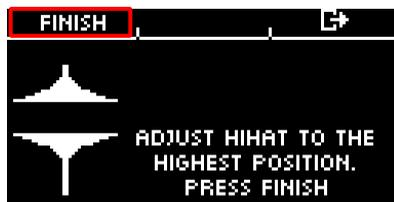
Now the hi-hat is fully calibrated and playable. With the hi-hat symbol you can directly test whether the mechanism works. Then confirm the setting by pressing the button **[F1]** „DONE“
