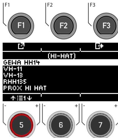
Select the **trigger** with the dial [5] or the navigation keys [8]. Confirm your selection with [F1] or by pressing [ENTER].
