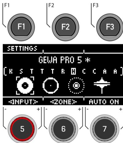
This **example** shows an activated bow components of Hi-Hat input.
