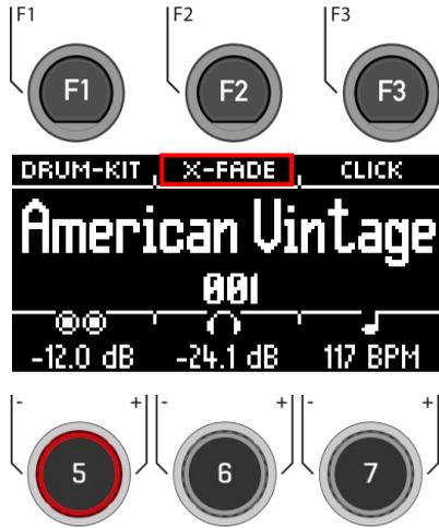
4. X-Fade EDIT = A window opens with a fader. Now you can set the threshold value that suits you with the dial [6]. The window closes automatically after 2 seconds.
