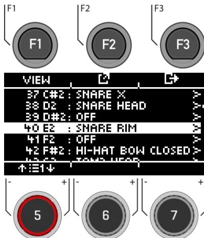
Use the control knob [5] or the navigation keys [8] to select the corresponding note.
