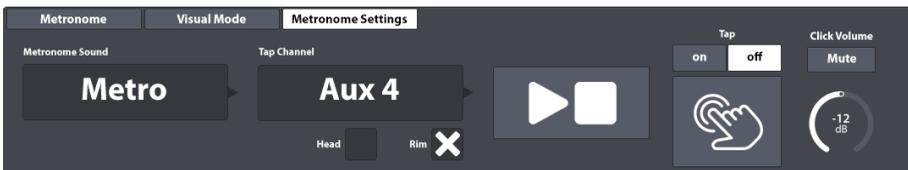
In this function set you can customize the **Metronome Sound** as well as the channel for setting the metronome speed by playing (**Tap Channel**).
