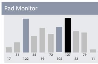
The pad monitor is useful for detecting whether a pad is maxing out at moderate strokes already, or a pad is causing barely audible double triggering.
