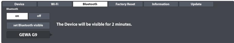
The built in Bluetooth function is useful for streaming music from an external player into the console. To establish a Bluetooth connection, you need to follow the steps below. Note that steps 2-5 take place on your mobile device and the procedure might vary from manufacturer to manufacturer. Please refer to the owner's manual of your mobile device if you have problems establishing a working Bluetooth connection:
