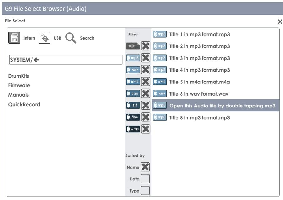
The **left column** displays all **folders** in the open directory, the **right column** lists all contained **files**. Double tap on a folder name to open it moving down the directory path. Tap on the **[white bar]** below the **[SD]** and **[USB]** buttons to move up the path by one node each tap. The **panel in the middle** contains **filter** options and **sorting functions**. Check the boxes as desired to display contents the way you prefer.
