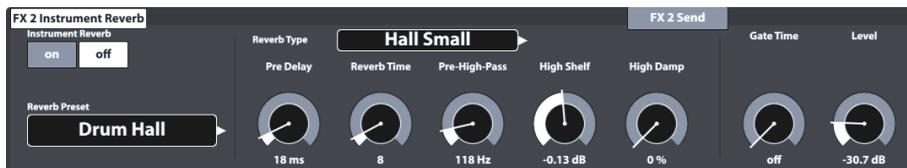
This module hosts classic and generic algorithms to simulate Instrument specific reverb. Some **Reverb Types** are traditionally generated electronically, whereas others (e.g. Plate) emulate mechanical devices designed to add artificial reverb to the dry recording.
