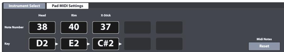
In this function set the user can set key values for **Midi OUT** configurations. **MIDI IN** signals regarding **trigger detection** of connected pads are fixed and can't be modified.
