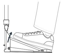
Release the pedal completely or remove the foot before tapping **[Calibrate]**
