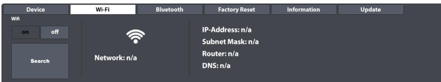
Within this function set you can manage all your Wi-Fi connections and settings. The Wi-Fi connection is essential to the use of the sound store online as well as the internal update function.
