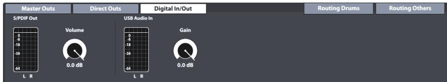
This function set controls the volume of the digital audio connections. Note that USB Audio can be used next to the occupation of the USB port as MIDI. Audio and MIDI Data can flow at the same time. The logarithmic faders allow for digital attenuation of signals within a range between  $-\infty$  dB (max) to 0 dB (min).
