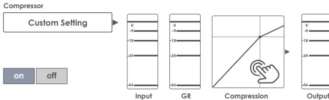
4. Set the **[Threshold]** for the Compressor to start working.
