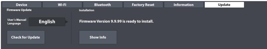
The Update section of the G9 derives its data from the default SYSTEM folder "Firmware" on the internal SD Card. All files contained meeting the criteria for check sums, naming conventions and version number will be considered. The latest valid firmware version will be provided for Installation. In that sense the update section operates as a firewall for defective and modified files.
