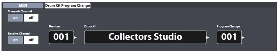
This feature set defines the rules for MIDI program changes. Since the G9 is a rhythm device, it can't be compatible with the standard MIDI protocol. The programs to change are the drum kits available in the **Drum Kit Browser**, where the **Drum Kit index number equals the program**.
