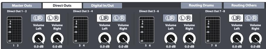
Adjustments of **Direct Outs** work in the same way as **Master Outs**, but with the exception that **Direct Outs** can be configured as either **Dual Mono** outputs or **Stereo** outputs. The choice in configuration will take effect in the routing matrix **Routing Drums** (see 12.1.4 *Routing Drums & Routing Others* on page 107).
