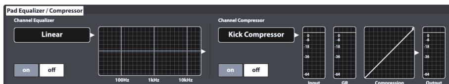
This function set hosts Equalizer and Compressor features which can be assigned to each Input channel displayed in **Module 1** of the **Kit Editor** Mode. Settings made in this module will be bundled with RAW MIDI signals and will consequently be audible in the direct outs when activated. (See also 12.1.4 Routing Drums & Routing Others on page 107)
